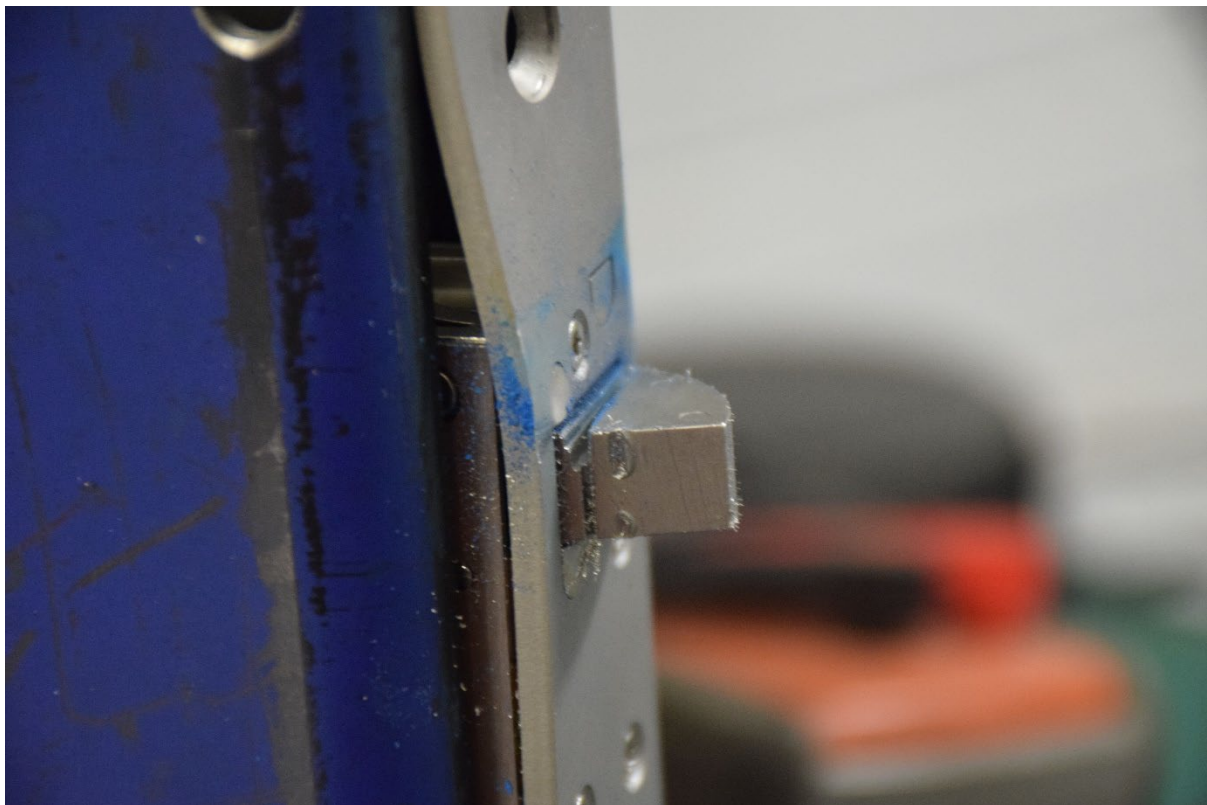
Figure 2: Showing both the faceplate deformation from C6.1 and the sawblade cut from C6.20
